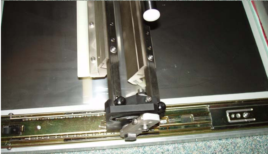
Attachment to manual screen printer. Adjusted pressure on stencil in both forward and backward prints.
